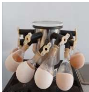
Figure 3 Drying of water extract by Freeze Dryer
