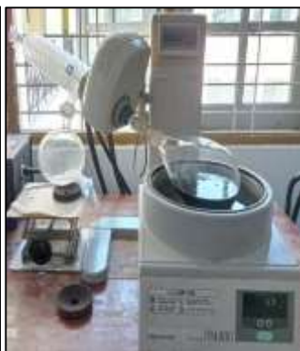
Figure 2 Removal of solvent by Rotary Evaporator
