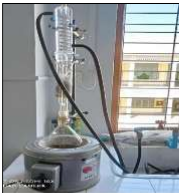
Figure 1 Extraction of leaves by Soxhlet
